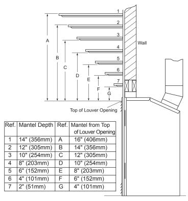
Figure 6 - Clearances for Combustible Mantels
